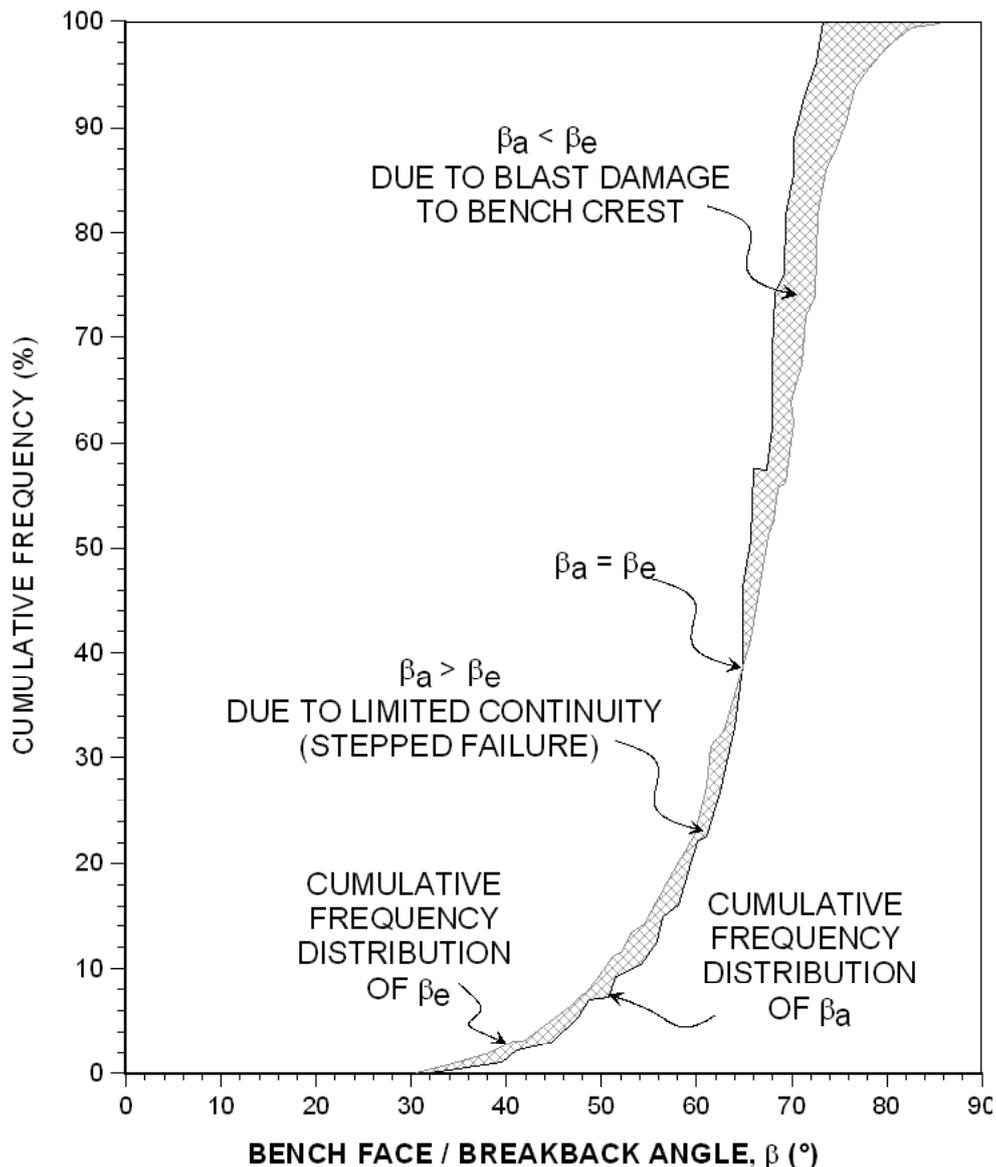
Figure 3 - As-built Bench Face Angle vs. Expected Breakback Angle
