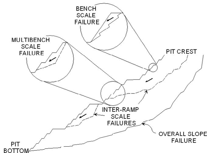
Figure 9 - Scale of Instabilities
