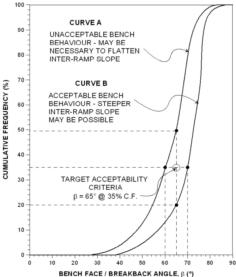
**Figure 4** - Assessment of Bench Performance Using Cumulative Frequency Analysis
