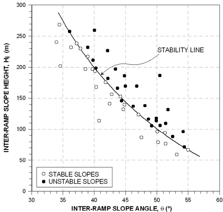
Figure 8 - Inter-ramp Height vs. Inter-Ramp Slope angle.
