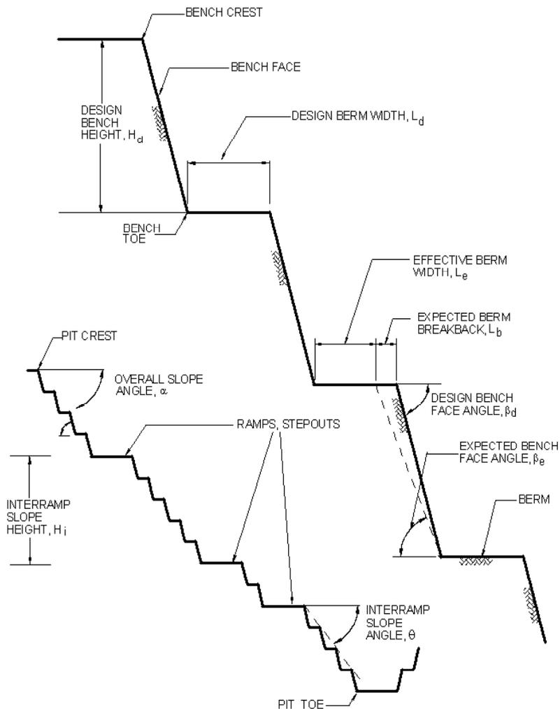
Figure 2 - Basic Slope Geometry Parameters
